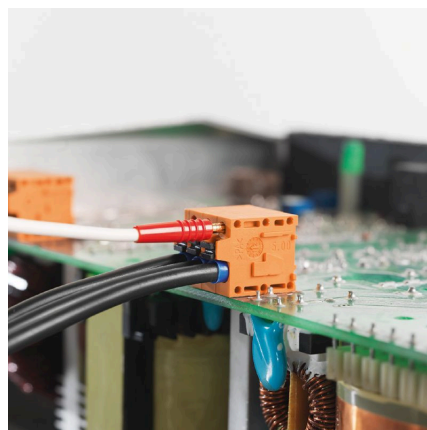
Maintenance through test point
