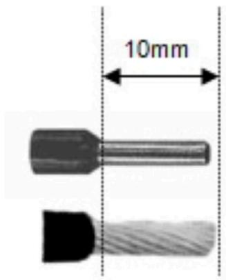
When using wire-end-ferrules, we recommend the length of 10 mm.
