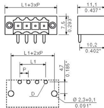
$L1 = 21.00 \text{ mm}$  |  $P = 3.50 \text{ mm}$
