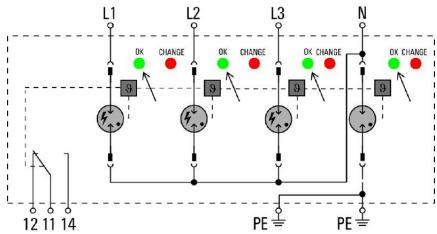
Schematic circuit diagram
