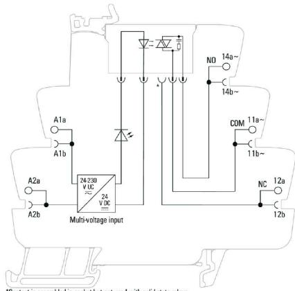
\*Contact is assembled in socket but not used with solid-state relays
