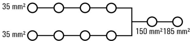
Conductor connection data according to IEC 60947-1 (Cu)
