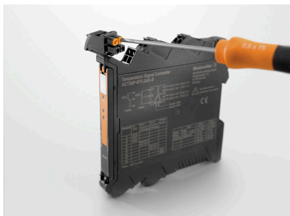
coding of terminal block
