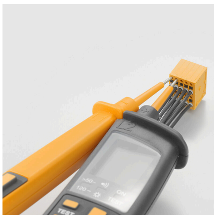
Maintenance through test tap
