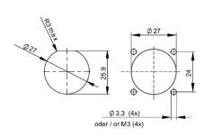
Mounting cut-out: 1. With central screw connection / 2. For mounting with four M3 screws
