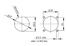
Mounting cut-out: 1. With central screw connection / 2. For mounting with four M3 screws
