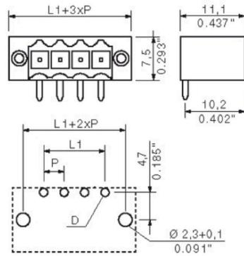
$L_1 = 17.50 \text{ mm} | P = 3.50 \text{ mm}$
