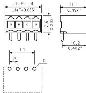
$L1 = 3.50 \text{ mm} | P = 3.50 \text{ mm}$
