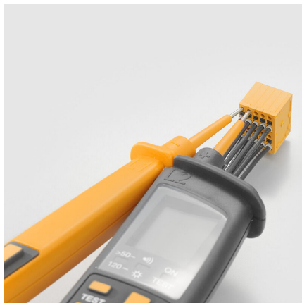
Maintenance through test tap
