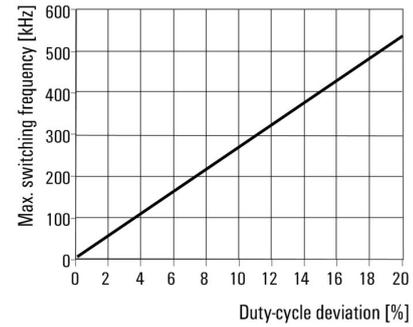
**Max. switching frequency depending on the duty-cycle deviation**
