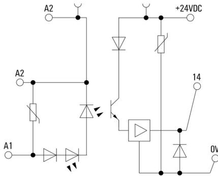
**Max. switching frequency is dependent on the duty cycle deviation**
