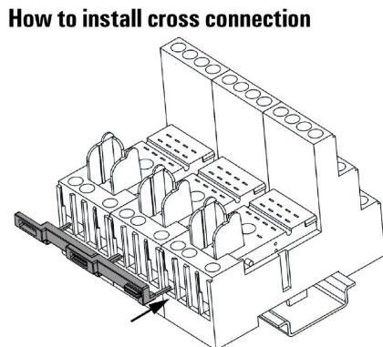
Plug the cross connection into wire-connection opening
