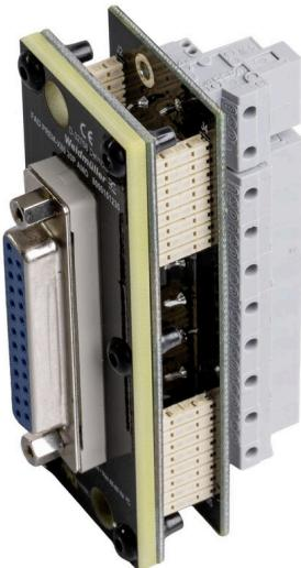
The Addcon adapters are installed on the new PLC. Just by plugging the old PLC cable to the adapter the migration is completed. No additional accessories (racks or cables) are needed.
