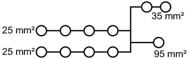
Conductor connection data according to IEC 60947-7-1 (Cu)
