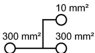
Conductor connection data according to IEC 60947-7-1 (Cu)
