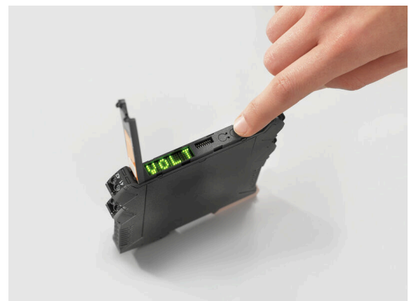
setting via display and push-buttons
