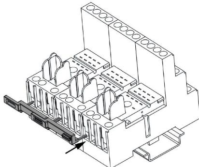
Plug the cross connection into wire-connection opening
