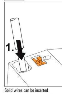
Solid wires can be inserted without opening the terminal.
