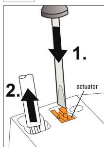
Push the actuator with a screwdriver to remove the wire.
