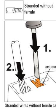
Stranded wires without ferrule can be inserted by pushing down the actuator using a screwdriver.
