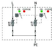
Schematic circuit diagram
