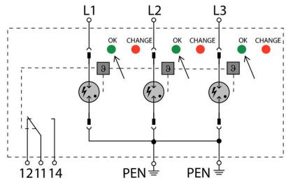
Schematic circuit diagram
