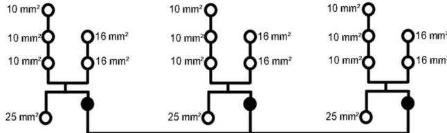
Conductor connection data according to IEC 60947-7-1 (Co)
