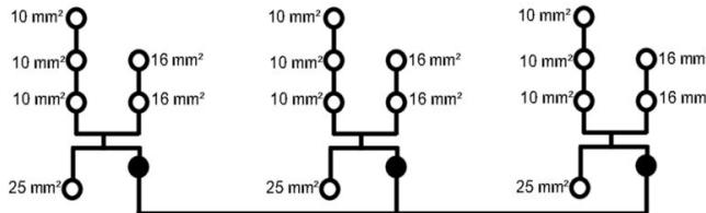
Conductor connection data according to IEC 60947-7-1 (Ce)
