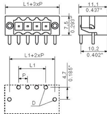
$L1 = 49.00 \text{ mm}$  |  $P = 3.50 \text{ mm}$
