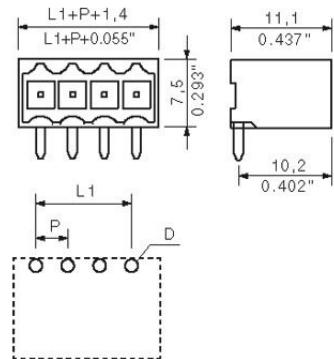
$L_1 = 10.50 \text{ mm} | P = 3.50 \text{ mm}$
