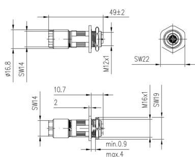
**Schema dei poli**
