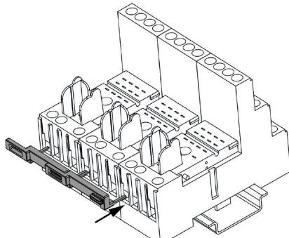
Plug the cross connection into wire-connection opening
