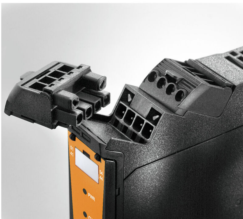
Removable terminals with coding
