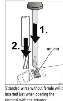
Stranded wires without ferrule will be inserted just when opening the terminal with the actuator.
