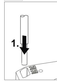
Solid wires will be inserted without opening the terminal.
