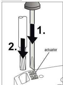
Stranded wires without ferrule will be inserted just when opening the terminal with the actuator.
