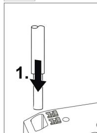
Solid wires will be inserted without opening the terminal.
