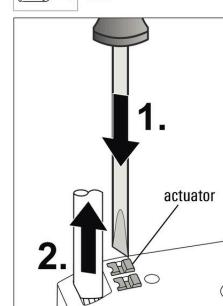
Wires will be disconnected just when opening the terminal with the actuator.
