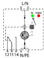
Schematic circuit diagram
