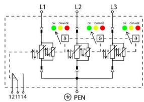
Schematic circuit diagram
