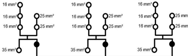
Conductor connection data according to IEC 60947-7-1 (Cu)
