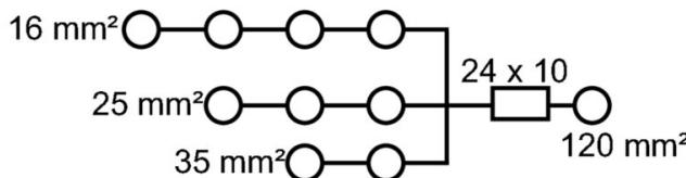
Conductor connection data according to IEC 60947-7-1 (Cu)
