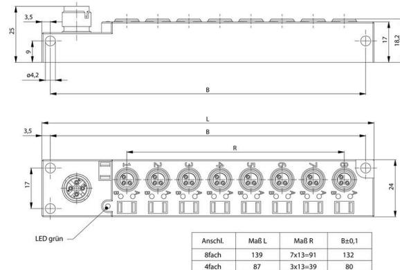
**Schéma****M8 | PIN 4**
