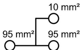
Conductor connection data according to IEC 60947-1 (Cu)
