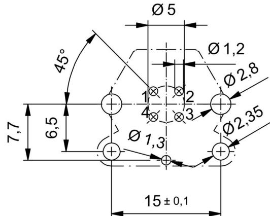
**Section de la face avant**
