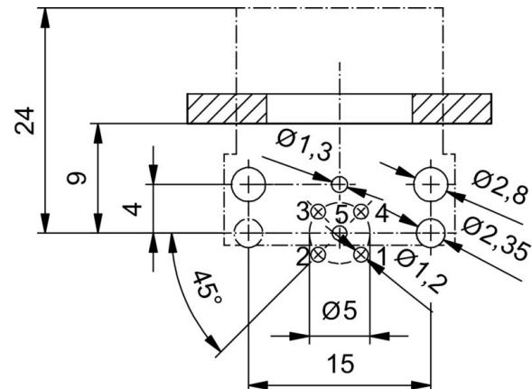
**Section de la face avant**
