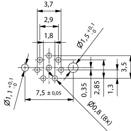
**Schéma des pôles**
