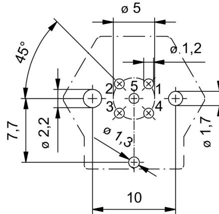
**Section de la face avant**
