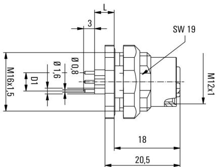
L(board-to-board distance) = 5,5mm D1 = 5,0 mm
