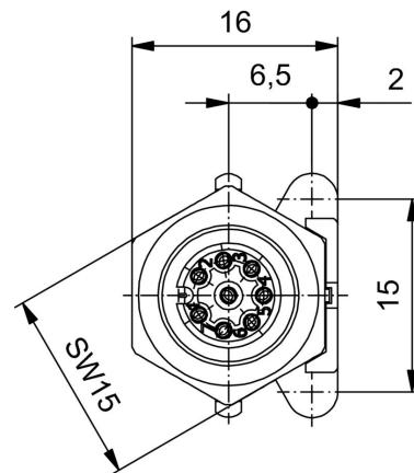
**Section de la face avant**
