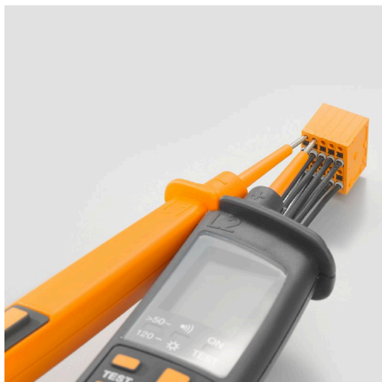
Maintenance through test tap
