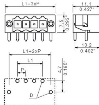
$$L1 = 38.50 \text{ mm} \quad | \quad P = 3.50 \text{ mm}$$
