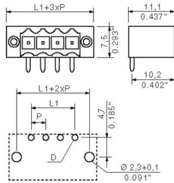
$L_1 = 80.50\text{ mm} | P = 3.50\text{ mm}$
