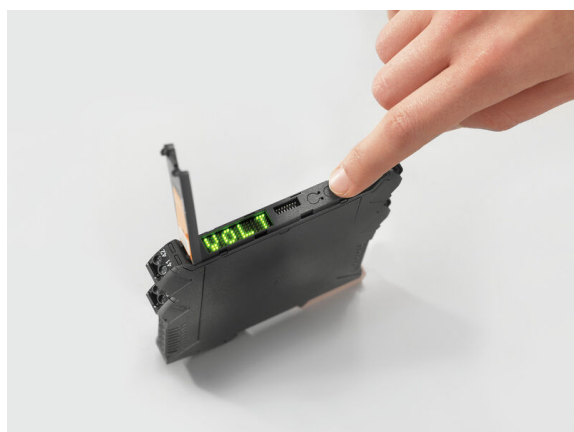
setting via display and push-buttons
