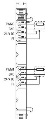
**Explication des abréviations****Pulse width modulation modules**
