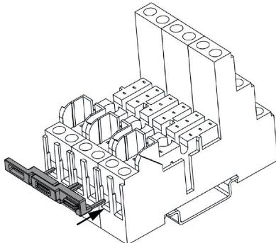
Plug the cross connection into wire-connection opening
