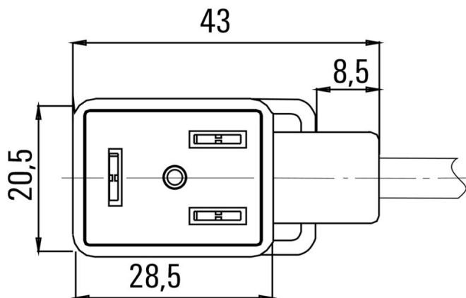
**Schéma des pôles**
